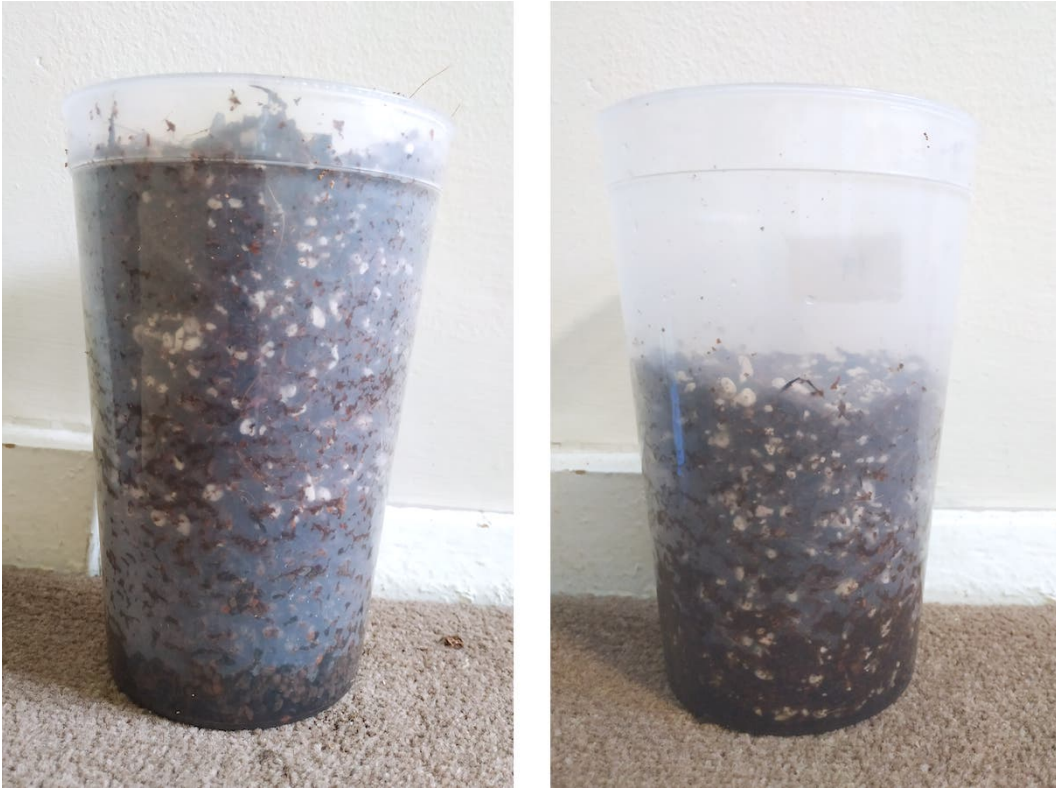
Figure A.1: Comparison of CPB medium with 60mm layer of grit (left) to CPB medium alone to a depth of 60mm below the top (right). In the left image, the perched water table in the medium is completely eliminated, and the low perched water table in the grit is visible.
