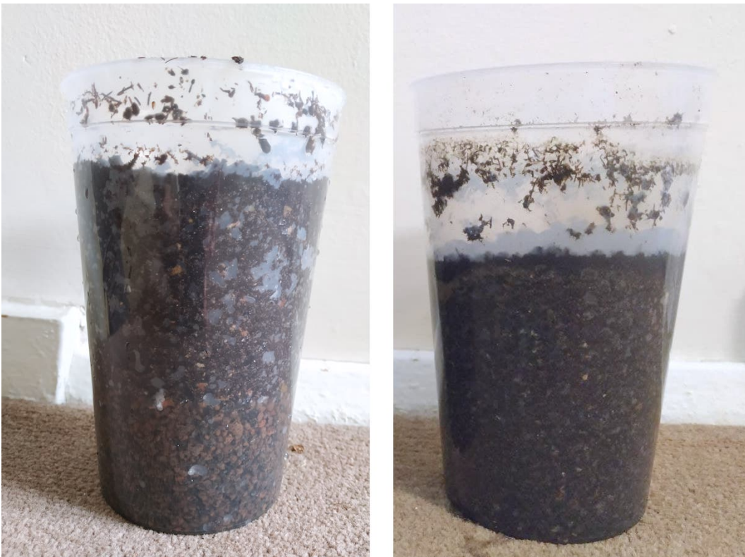
Figure A.2: Comparison of JI medium with 60mm layer of grit (left) to JI medium alone to a depth of 60mm below the top (right). In the left image, the grit layer appears to be completely saturated after drainage.
